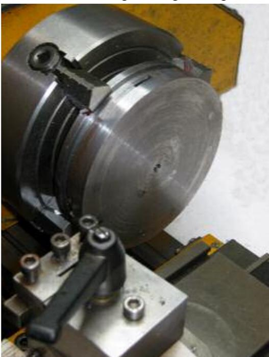
The work was reversed in the 4-jaw and I mounted my Headstock Dividing Attachment on my lathe so I could make the 360 divisions around the lower part of the table – right photo and below.
