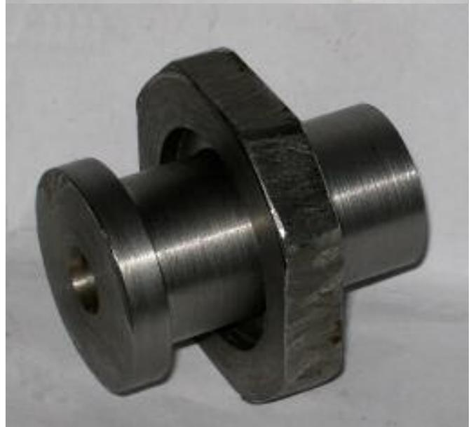
After silver soldering (brazing) and pickling the work was mounted between centres and turned slightly oversize. The flange was turned to dimension on the outside and faced to just under 5mm thick – right photo.
