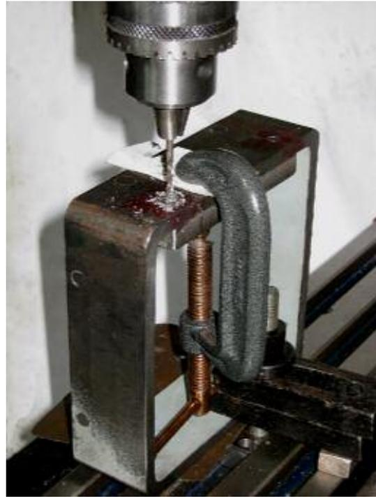
The slots were milled with an 8mm slot drill to a depth of about 8mm – left photo.
