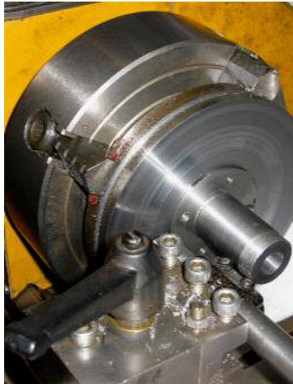
and the spigot turned to 25mm for a push fit in the ball bearing. The rest of the spigot not being "occupied" by the ball bearing was turned down slightly to a sliding fit in the hub that will carry the wormwheel, and slightly more at the very end where a 1.5mm pitch thread was cut for the nut that adjusts axial play.
