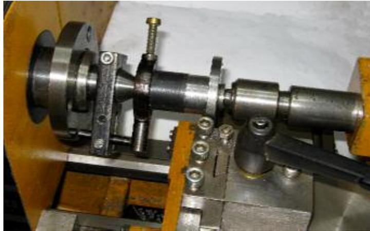
The bottom part of the table was mounted in the 4-jaw and centred, one side faced. Then turned around and the other side faced and the groove was cut using a parting off tool.
