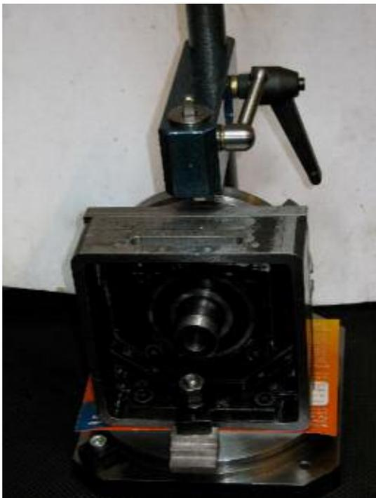
mount the table on the base and mount the hole on the milling machine table and mill the upper part of the T slots using a 10mm slot drill. A slot drill might not produce as accurate a slot as a slot drill, but I wanted the slot slightly wider than 10mm so I took a light cut along each side after cutting the slot. I had made a simple Pillar Tool inspired by the one George Thomas made and used that to punch the numbers – left photo.
