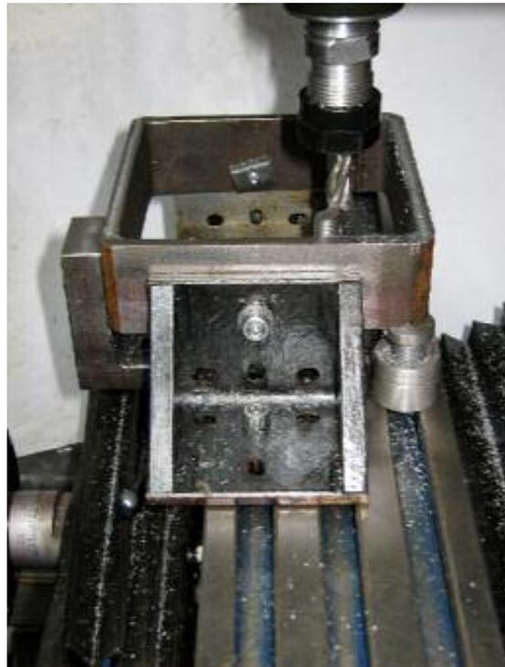
Since the square tube was thin walled (about 4mm) I had to screw and solder 4 pieces of steel at the top of each corner. The joints were fluxed and with the screws tight the four pieces were silver soldered (hard soldered) to the tube, just beneath the top surface.
