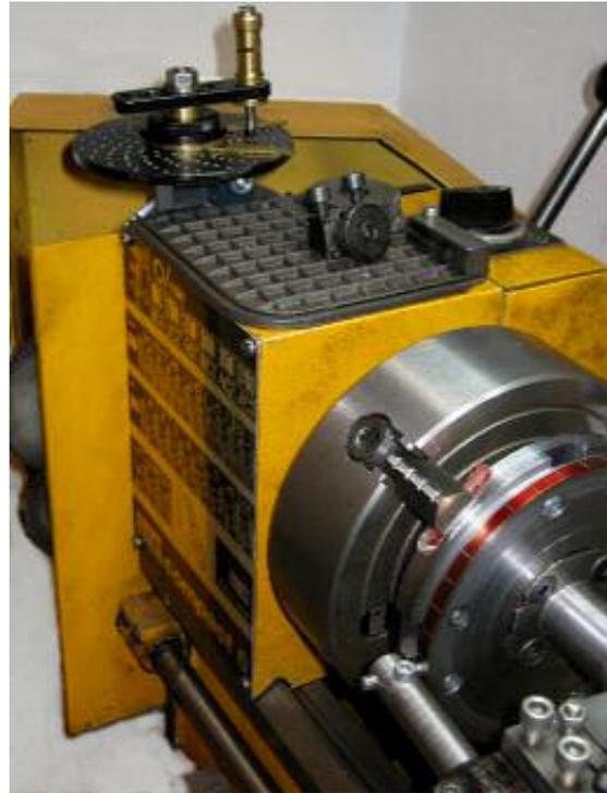
I just mounted a V shaped tool in my boring bar and used a carriage stop to get the length of the divisions correct. I marked the 36 ten degree marks first, then the 5 degree arcs slightly shorter and so on. The result is shown in the upper left photo.
