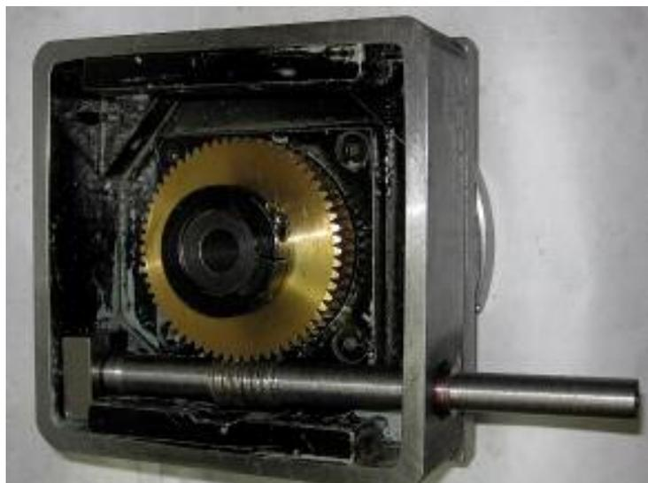
M4. Since the holes in the bearing housing are oversized it is possible to make small adjustments and take up wear in the worm and wheel.
