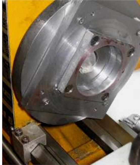
This is how it looks after the Table Bearing Housing is finish turned and bolted and glued to the Base Top Plate and the Base assembled, with the ball bearing mounted and the inside given a coat of primer.
