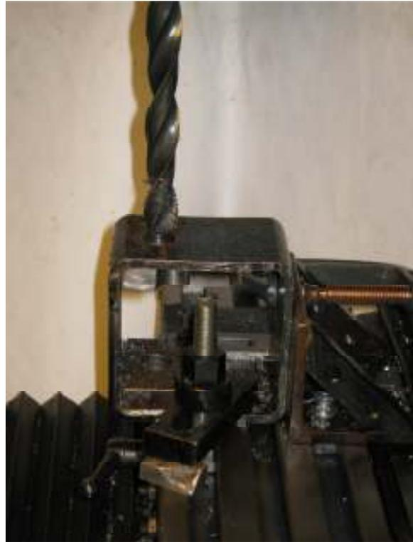
The photo to the right shows the crankshaft and bearing mounted on the base. A couple of oil-holes are visible on the top.
