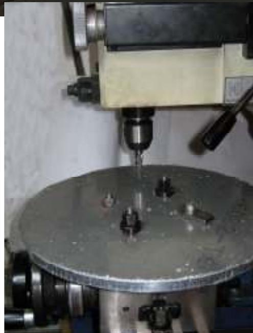
the work and the table) on my rotary table and mill the outer part circular.
