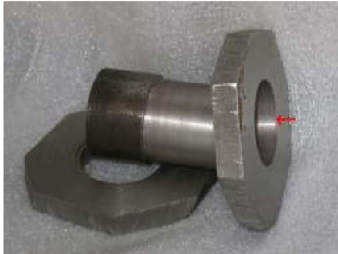
In fact I made two identical hubs since I needed a countershaft to get the speed reduction needed.
