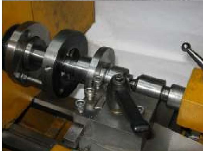
I did struggle to find a second large pulley for the countershaft, but after a while a friend got me a large PolyV pulley that I could mount on the second hub. For the countershaft I used another piece of the 80mm square steel tube, but instead of Oilite bushes I used two 20mm Pillow Block ball bearings. The countershaft will rotate at a higher speed than the crankshaft. I also turned a small diameter PolyV pulley for the motor. I must find some material to make some belt and pulley guards.
