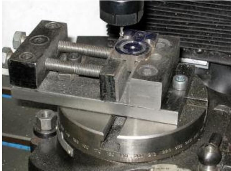
The hand-wheel dials on the milling table was used to place the cutter 7.5mm from the centre of the 4mm pivot hole when milling the steam channels, and the 17.5mm distance to the 2.5mm hole that will be tapped M3 for a screw to hold the Little End of the *Eccentric Rod*.
