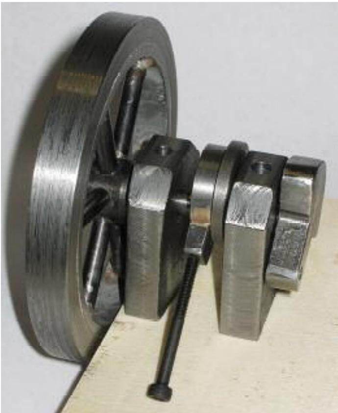
Here is a photo of the *Flywheel*, *Bearing Blocks* and *Eccentric* mounted on the *Crankshaft*. I just put a long M3 screw in the *Eccentric Strap* so it wouldn't rotate when I turned the *Flywheel*.
