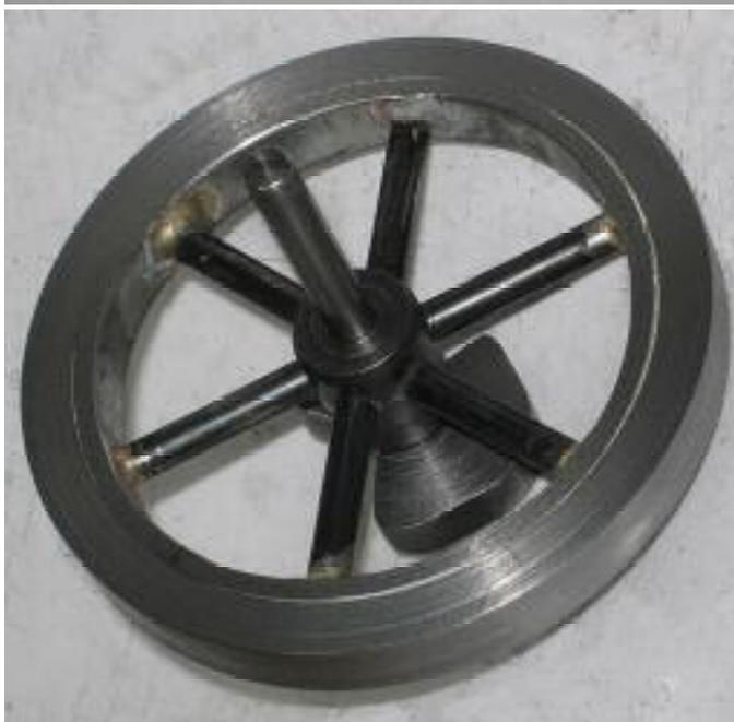
was mounted on a tapered mandrel between centres and the outer diameter and sides finish turned to remove some wobble, well most of it. The thick-walled tube used for the outer ring should have been a bit wider, but I used what I had at hand.
