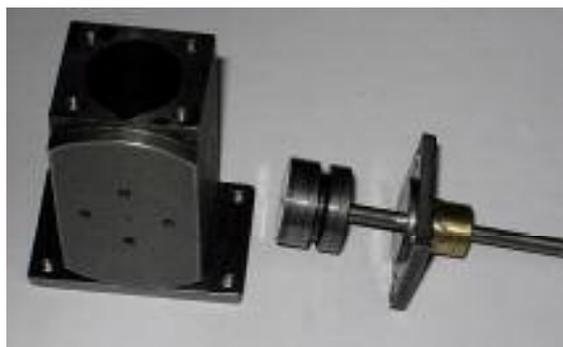
parted off side faced. The *Piston* with *Piston Rod* was then turned to a nice fit in the *Cylinder*. The *Piston Rod* was made from a piece of 1/8" free-cutting stainless steel, the M3 thread on the end was cut in the lathe.
