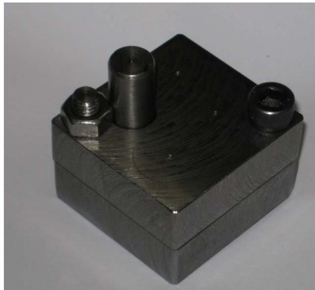
A drilled hole isn't perfectly round so for the large holes I mounted the two parts in the 4-jaw. I first drilled an undersize hole and then bored the hole to dimension, this gave a better result.
