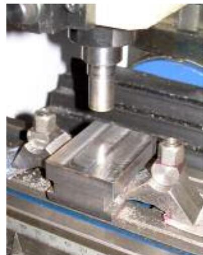
The position of the V was marked on the block. I used an angle vise to clamp the block in a 45 deg. position so I could mill the V.
