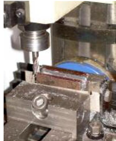
The top and bottom of the work was fairly flat from the manufacturing process. With the two slots milled the work was clamped directly to the mill table and the top and bottom surfaces cleaned up with a carbide tipped end mill. This will make the top and bottom surfaces parallel with each other. The surface of HRS is hard and will soon dull a HSS end-mill, carbide is much harder.
