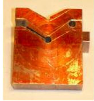
Two clamps were glued together with superglue and machined together. I used M5 allthread and machined M5 nuts (see picture below).
