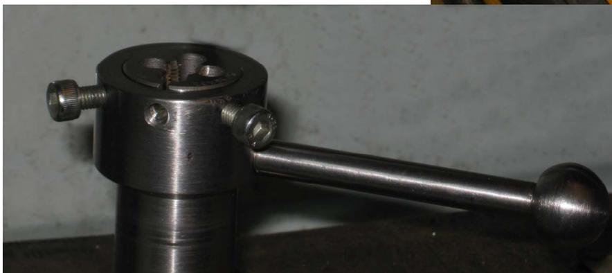
I have also got a smaller die – 13/16" – so I made a die holder for this. This time I used a piece of rod from my scrap box and just drilled a 10mm through hole so I can use a 10mm rod in the tailstock drill chuck to support the die holder.
