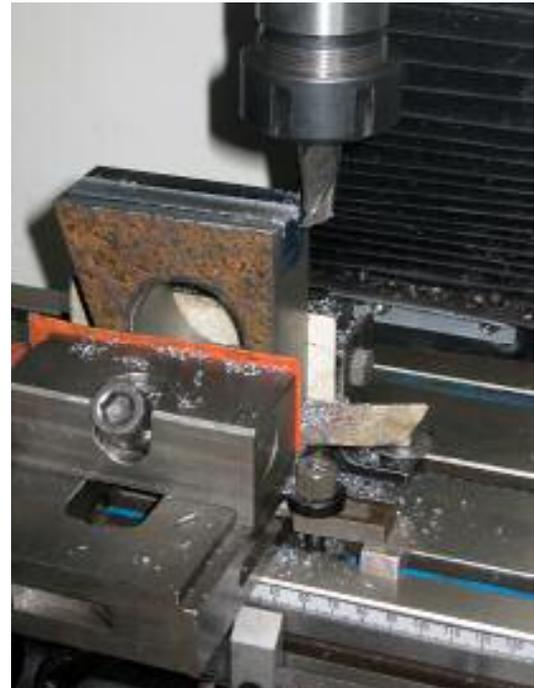
Then I drilled a 6.8mm hole close to the end opposite the slot. The 6.8mm hole was opened up to 8mm for a little over half the length, the 6.8mm part of the hole was then tapped M8. I then used a hacksaw to make a cut from the outside and in to the 40mm hole so the M8 bolt could clamp the tool-holder to the post.
