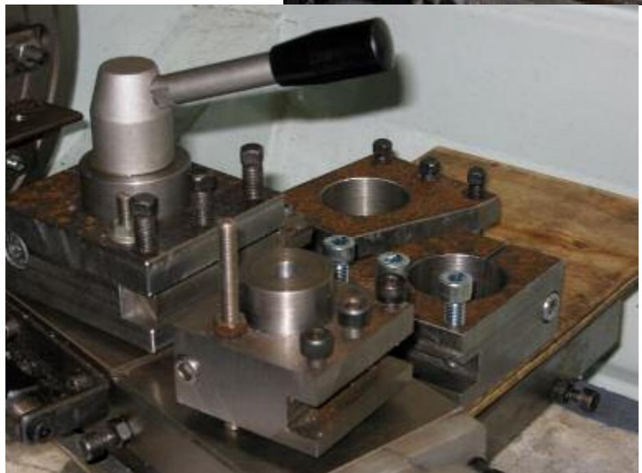
Here is a photo of two of the tool-holders after painting, one is mounted on the topslide, the other on the rear toolpost.
