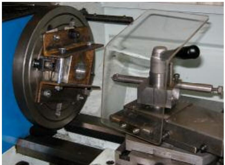
After boring the 40mm hole to a sliding fit on the toolpost the work was mounted in the milling vice so I could cut a slot for the lathe tools. My 290 lathe can take tooling with 13mm shanks so I decided to use a 14mm slot drill to mill the slot to a depth of 14mm – right photo.
