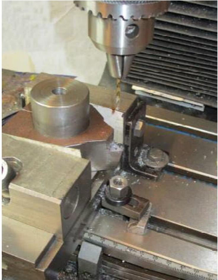
I also drilled a 5mm hole and tapped M6 for a height adjustment screw.
