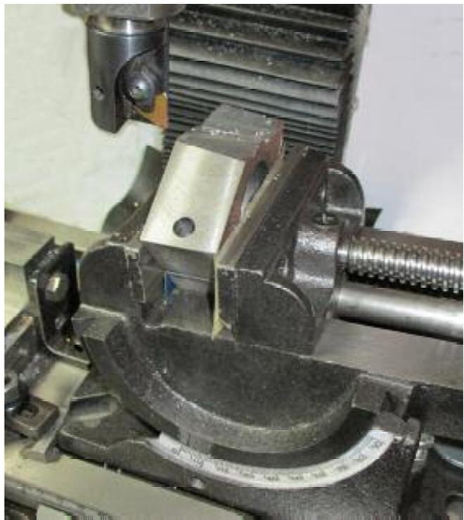
The tool-holder was mounted in the milling vice and I milled a step for the tungsten carbide insert. The insert was put in place and the hole for the clamping screw marked out. I didn't have a M2.5 screw so I tried to put a countersunk M3 Allen screw through the hole in the insert, and the hole was wide enough to let the screw pass. So I drilled a 2.5mm hole and tapped M3 – right photo.
